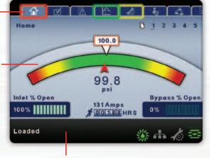
The compressor's most critical information is constantly displayed on the controller's status bar.
