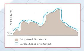
Nirvana control is delivered by a variable speed drive. The Nirvana 7.5-40 hp VSD maintains a close controlled system pressure, automatically adjusting its output to achieve the highest efficiency for your operation.
