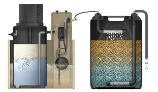
The key to the PolySep's performance is the specially coated Zeolite adsorption media
